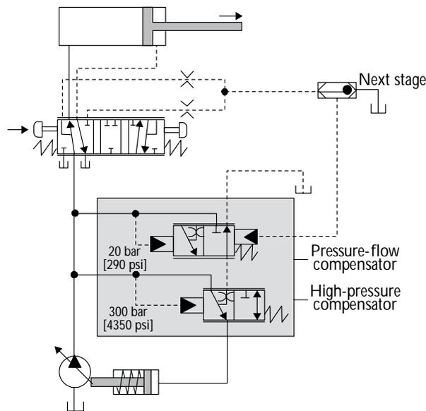
The load sensing system in the high-pressure stand-by mode
