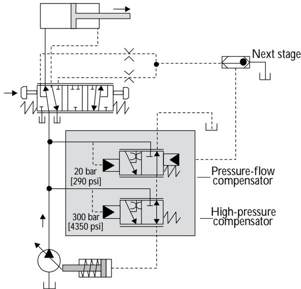
The load sensing system in the load sensing mode
