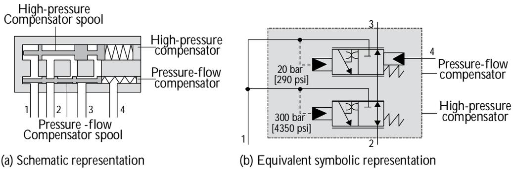
Schematic and symbolic representations of a pump compensator in a load sensing hydraulic pump
