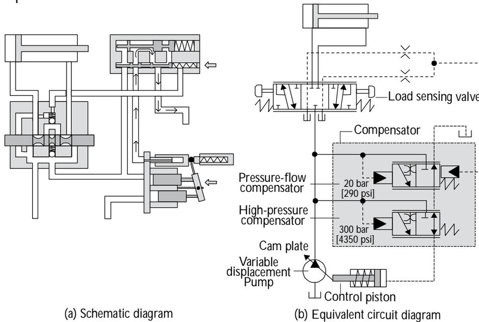
Schematic and symbolic representations of a simple load sensing system in its initial position
