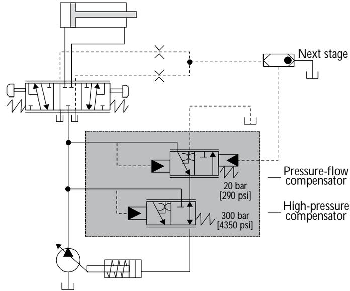
The load sensing system in the low-pressure stand-by mode
