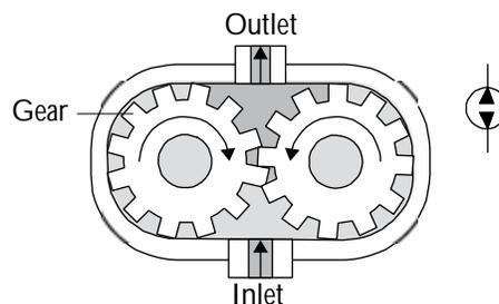
The gears rotate in opposite directions. They mesh at a point between the inlet and outlet ports to provide a tight sealing. The diverging teeth at the inlet create a partial vacuum, which draws fluid. The trapped fluid then travels around the periphery of the gears as two streams. As the pump has a positive internal seal against the leakage, the fluid is positively ejected out of its delivery port. The pump displaces a fixed volume of fluid in one revolution and creates the flow.
