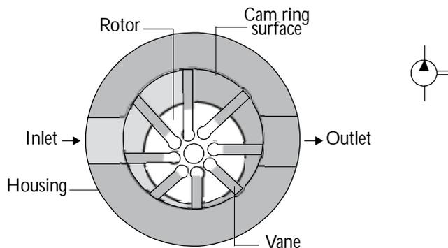
As the rotor rotates, the space between any two successive vanes at the suction side increases. This expanding volume creates a partial vacuum, which draws fluid into the chambers formed by the vanes. The fluid is trapped in these chambers, and it is then moved through the pump by the rotating vanes. As the space between the two rotating vanes decreases, the fluid is squeezed out through the discharge port and the pump creates the flow.
