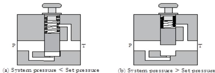
The operating characteristics of a direct-acting PRV are affected by the extent of non-linearity of its spring and any back-pressure on its discharge side.
