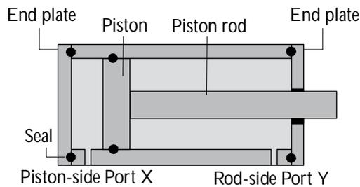
It is designed with either spring-assisted fast retraction or controlled retraction. If the system fluid is pumped into the piston chamber through the port X and the fluid in the piston-rod chamber is discharged through the port Y, then the piston-and-rod assembly extends with a definite force (thrust). A reciprocating linear motion can be obtained quite easily.
