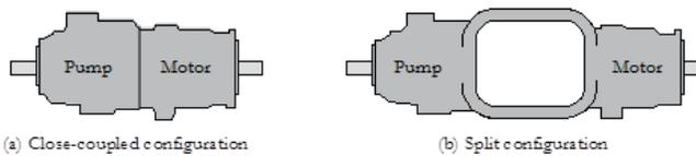
In the split configuration, the power unit with a hydraulic pump, heat exchanger, filters, valves, and controls is mounted on the reservoir, and a remotely mounted hydraulic motor is connected to the power unit through hoses or steel lines. The split configuration is typically used in heavy-duty applications because it offers full flexibility in configuring the system.
